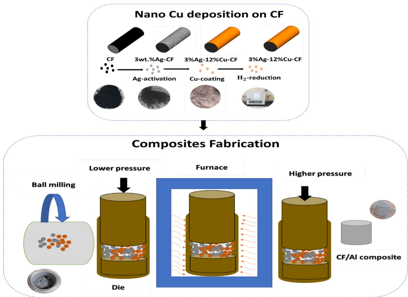
Fig. 2 Schematic illustration demonstrating the steps for preparing CF/Al composites
